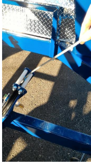
Figure 2. Repositioning the Auto-Bungee® Cable
