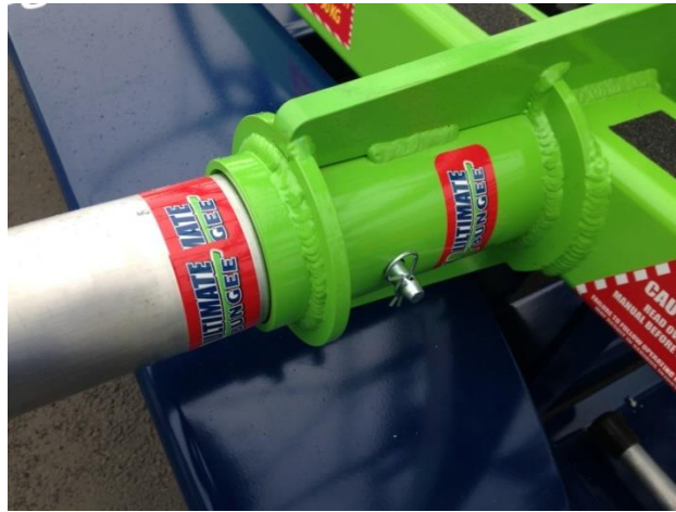
Figure 8. Matching the Aluminum Poles to the Mount
