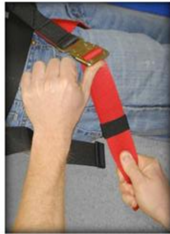
6. Tighten firmly by pulling on the webbing end, while making sure that it stays in the elastic loop.
