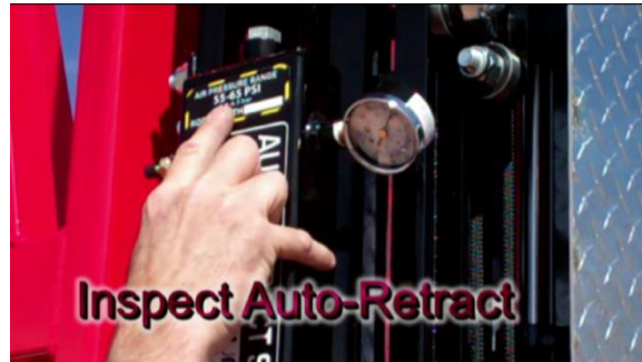
Figure 28. Check the Auto-Retract Pressure
