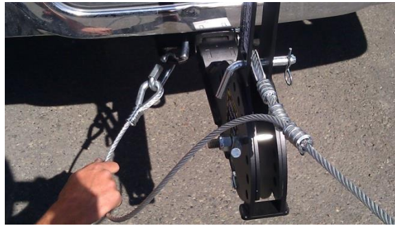
Figure 20. Connected ATD Cable
