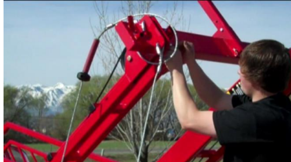
Figure 6. Loop Cable Around Mast
