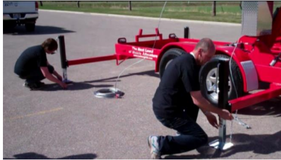
Figure 9. Adjust the Jacks
