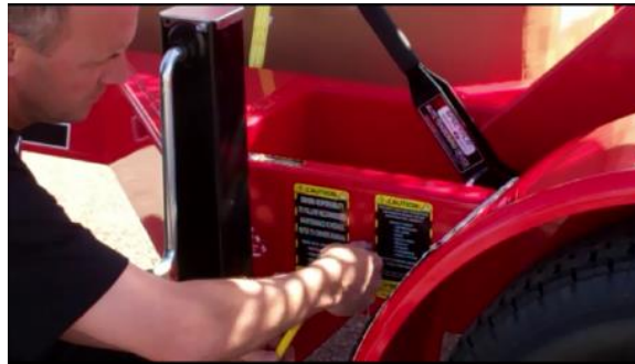
Figure 8. Use the Pendant to Raise the Tower
